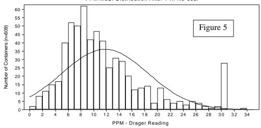
PPM MeBr 1-hr After Re-seal Following an 8-24 hr Aeration.
