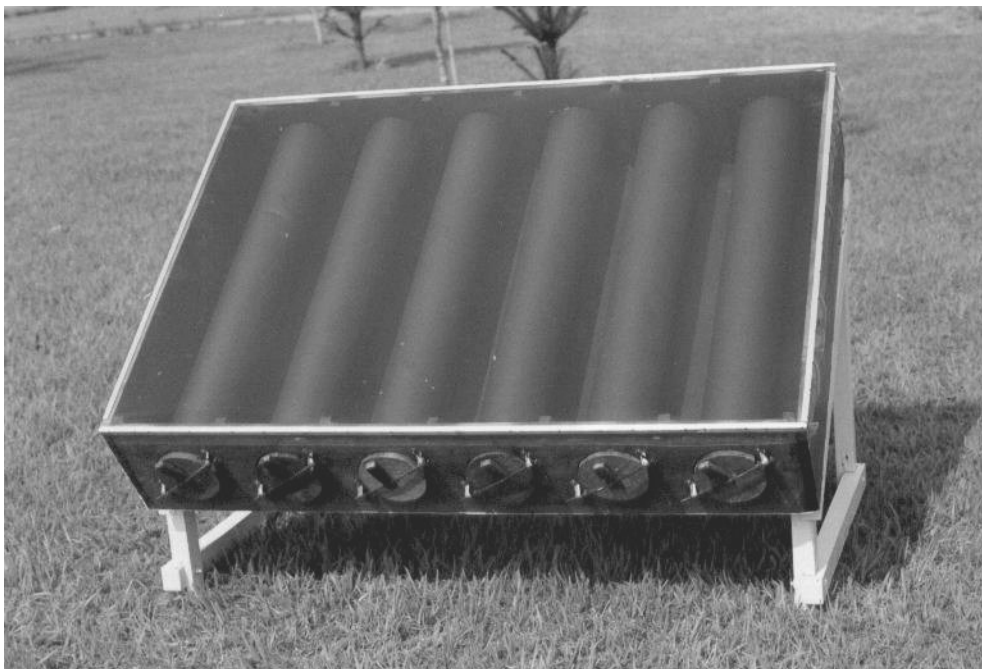
Fig. 1. Solar collector for substrate disinfestation.
