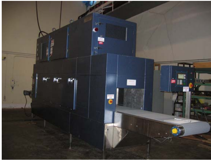
Fig. 1. A 27.12 MHz, 25 kW RF unit for large-scale tests
