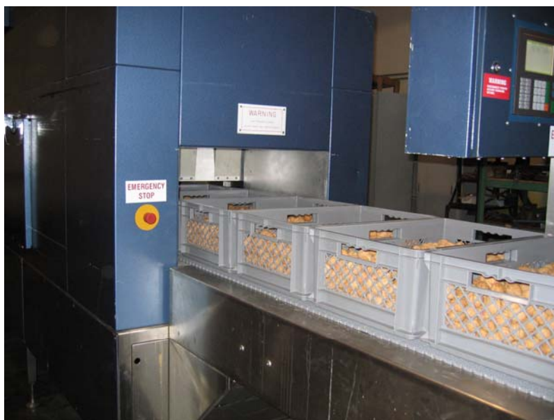
Fig. 3. Continuous process of RF treatment on inshell walnuts
