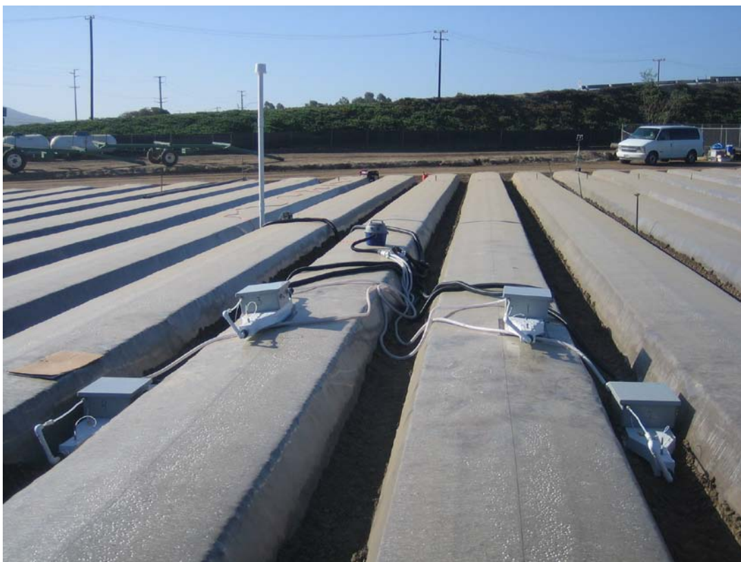
Figure 3. Field application of the Dynamic Flux Chamber System for measuring fumigant emissions.
