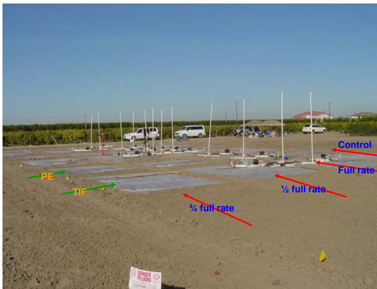
Figure 1. A field layout testing the effect of TIF tarp on emission reduction and efficacy from deep shank injection of Telone C35 in October, 2009 at Parlier, CA.
