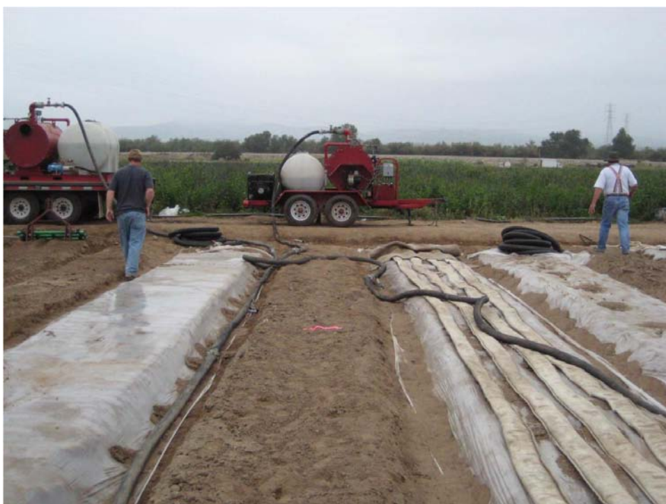
Figure 1. Steam applications in a cut flower nursery near Oxnard, CA in June 2010. Steam generated through either a propane- or diesel-fired boiler (background) is applied through buried drain tile (left) or through spike hoses inserted into bed tops (right).
