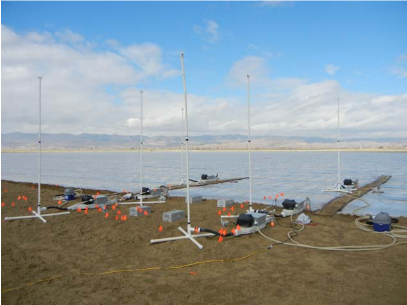
Figure 1. Sampling layout for emissions with dynamic flux chambers at TIF tarped and edge areas in a large field trial in June 2011, Lost Hills, CA.
