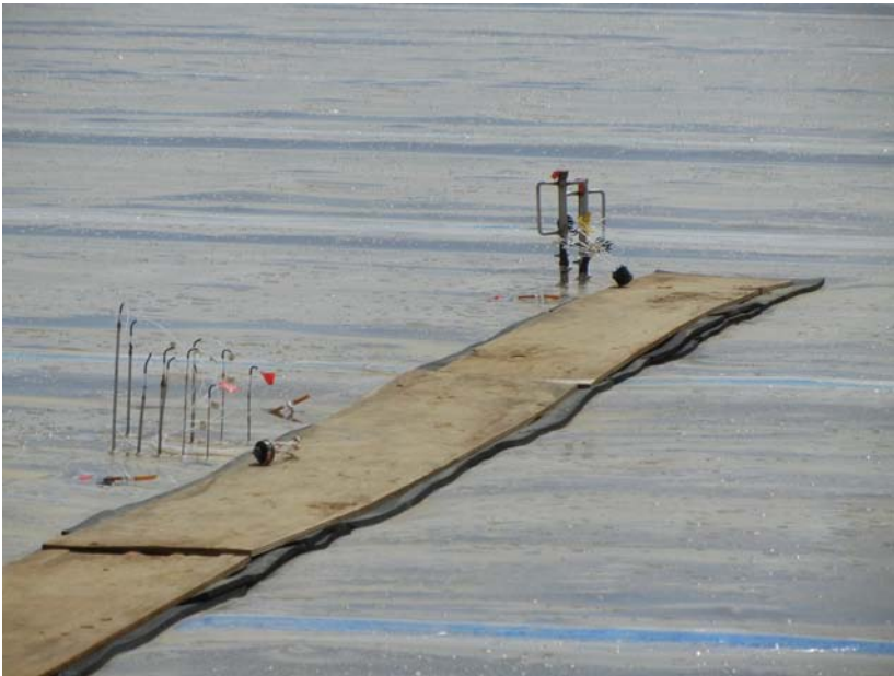
Figure 2. Soil-gas sampling probes for monitoring fumigant concentration changes in soil profile in a large field trial in June 2011, Lost Hills, CA. Probes were installed to various soil depths.
