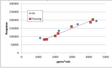
The SPME response to passively sampling a flowing system is the same as when sampling vial headspace.
