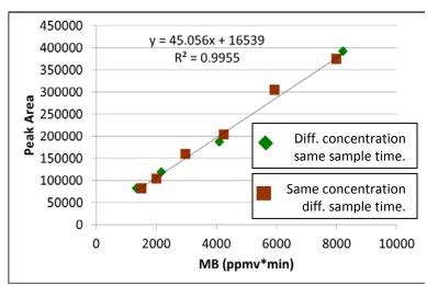
When the SPME fiber is not directly exposed to the sample stream, the amount of MB adsorbed is proportional to exposure (CxT).
