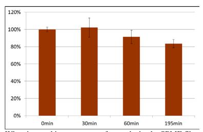
When inserted into a septum after analysis, the SPME fibers can be stored for up to 60min before analysis with no loss of quantitative information.
