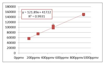
When used for active sampling, SPME fibers show linear response to methyl bromide and a several orders of magnitude signal enhancement over direct sampling of the air.
