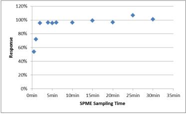
The fibers reach equilibrium with the concentration of MB in the air in ~2min.
