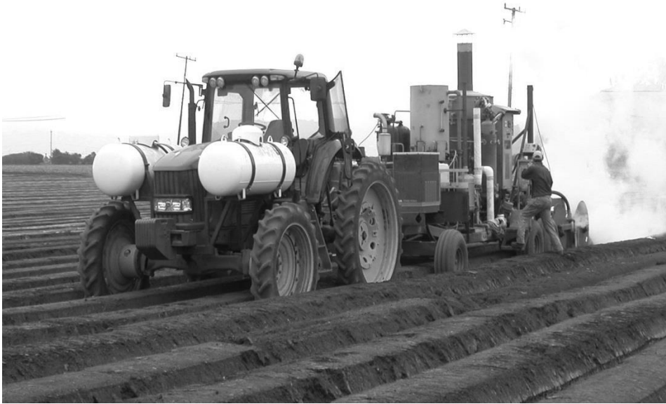
Figure 1: Tractor towed steam soil disinfestation machine prototype with Clayton 100 HP steam generator (Watsonville, CA Sept. 2012).
