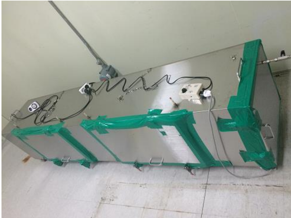
Figure 1. Designed mini shipping container(0.5 x 0.5 x 2.3m, stainless steel)
