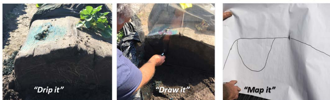
Figure 2. The first step in evaluation process of the drip stakes is to define what is the Treated Zone using a water soluble blue dye mixed into the drip water and measuring stained wetting area after.
