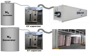
Liquid EF is vaporized with heated  $N_2$  gas through the nitrogen heater, which fitted in vaporizer and discharged through the fumigation chamber.
